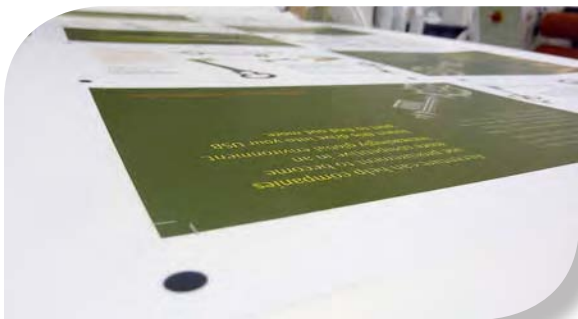
Printed registration marks and optical alignment ensure the cutting is perfect every time
