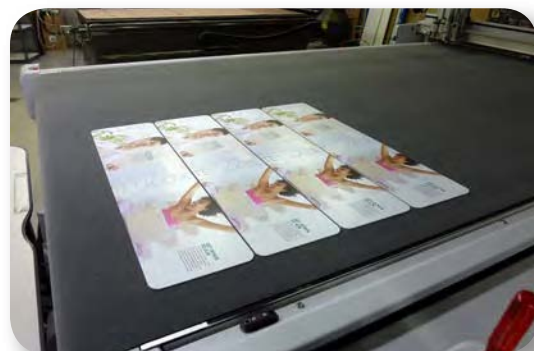
Panels being cut on CNC digital router
