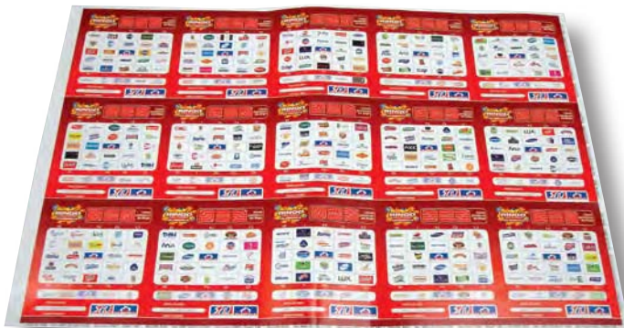
12"x18" press sheet with 450 random images driven by variable-data list
