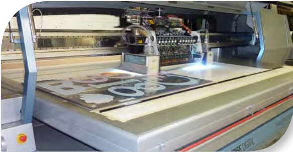
UV flatbed printing with opaque white ink
