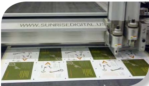
Cutting is done in multiple passes using different tools optimized for each material
